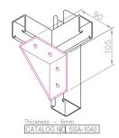
Standard Materials : Rolled Steel ASTM A36 Standard Finishes : Hot Dip Galvanized
