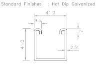
Standard Materials : Rolled Steel ASTM A36
